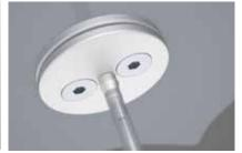
The air pressure measurement adapter enables the connection of a hose to air filled cushions to measure the inside pressure.
